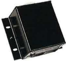
The Digital Input/Output (DI/O) module serves to provide expandable Input and Output event capability of the EMCP 4 and is capable of reading 12 digital inputs and setting 8 relay outputs.
