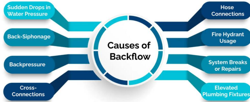
Figure 17: Diagram depicting several causes of backflow in a potable water supply.
